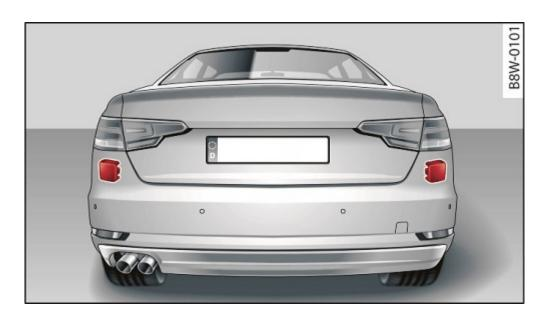
The radar sensors (marked here in red) are normally located in the rear area of the bumper cover. Please check for the exact location of the sensors in the workshop manuals e.g. Body repairs or Electrical system.
