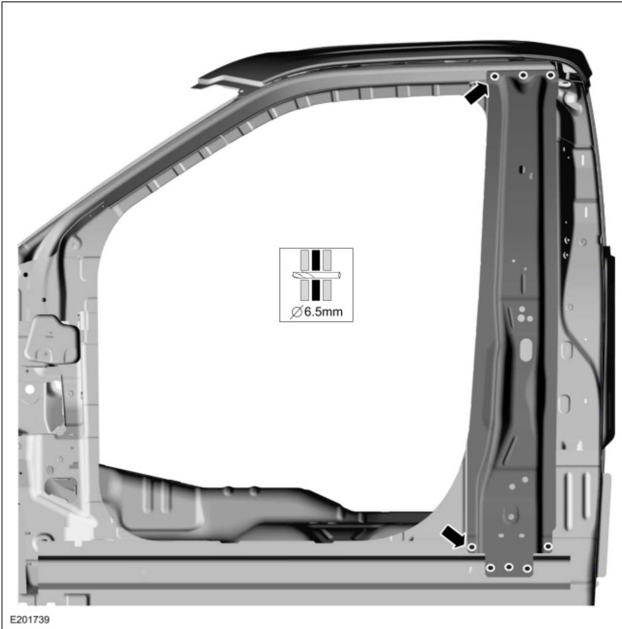
11. Install blind rivet fasteners.
