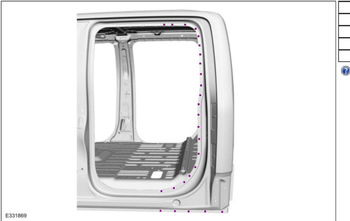
18. **NOTICE: Body side sectioning is prohibited within 50mm of door hinge, door striker and restraints anchoring points.**
