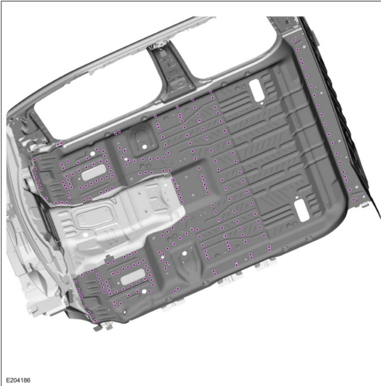
13. Remove the cab back to floor panel SPR fasteners.
