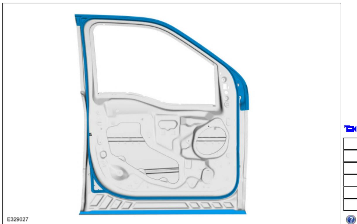
9. Remove the seam sealer from the door hem flange.
