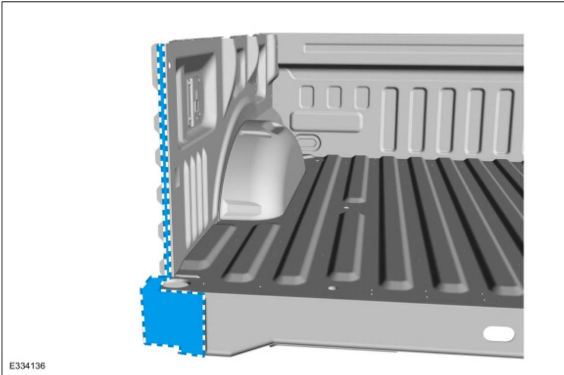
3. Install the pickup box corner reinforcement and clamp in position.
