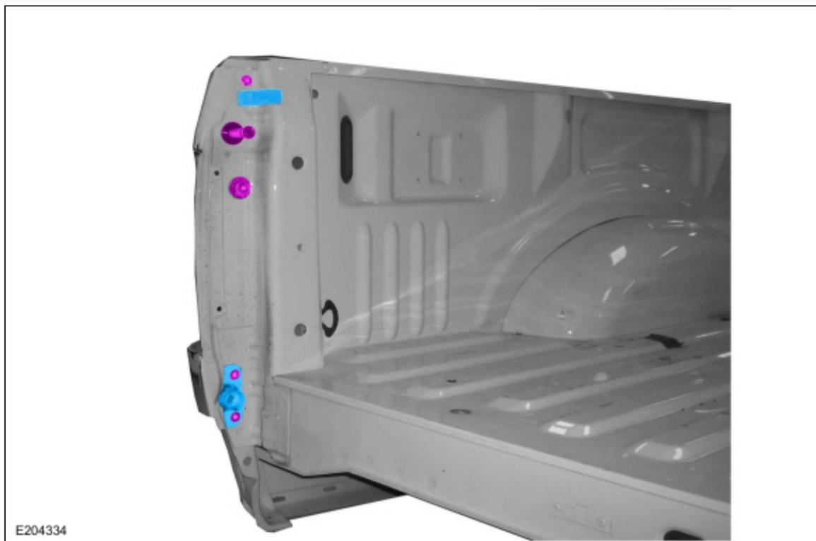
6. Route the tail lamp wiring harness out the bottom of the reinforcement and position aside.
