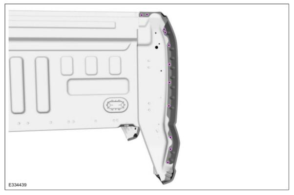
12. Remove the <u>SPR</u> fasteners.
