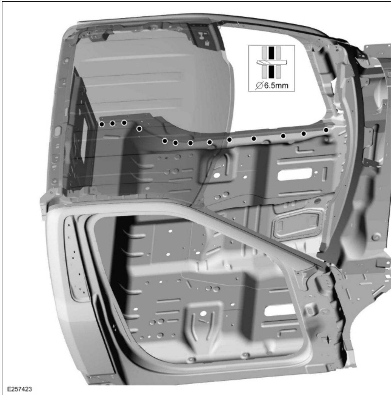
6. **NOTE:** *Blind rivet or solid rivet fasteners may be used in place of SPR fasteners after enlarging holes to 6.5 mm.*
