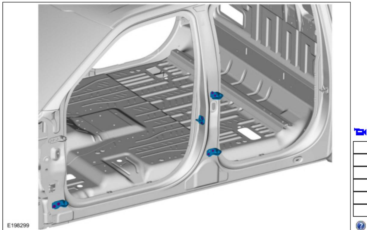
30. Install the front and rear door opening weather strips and scuff plates.
