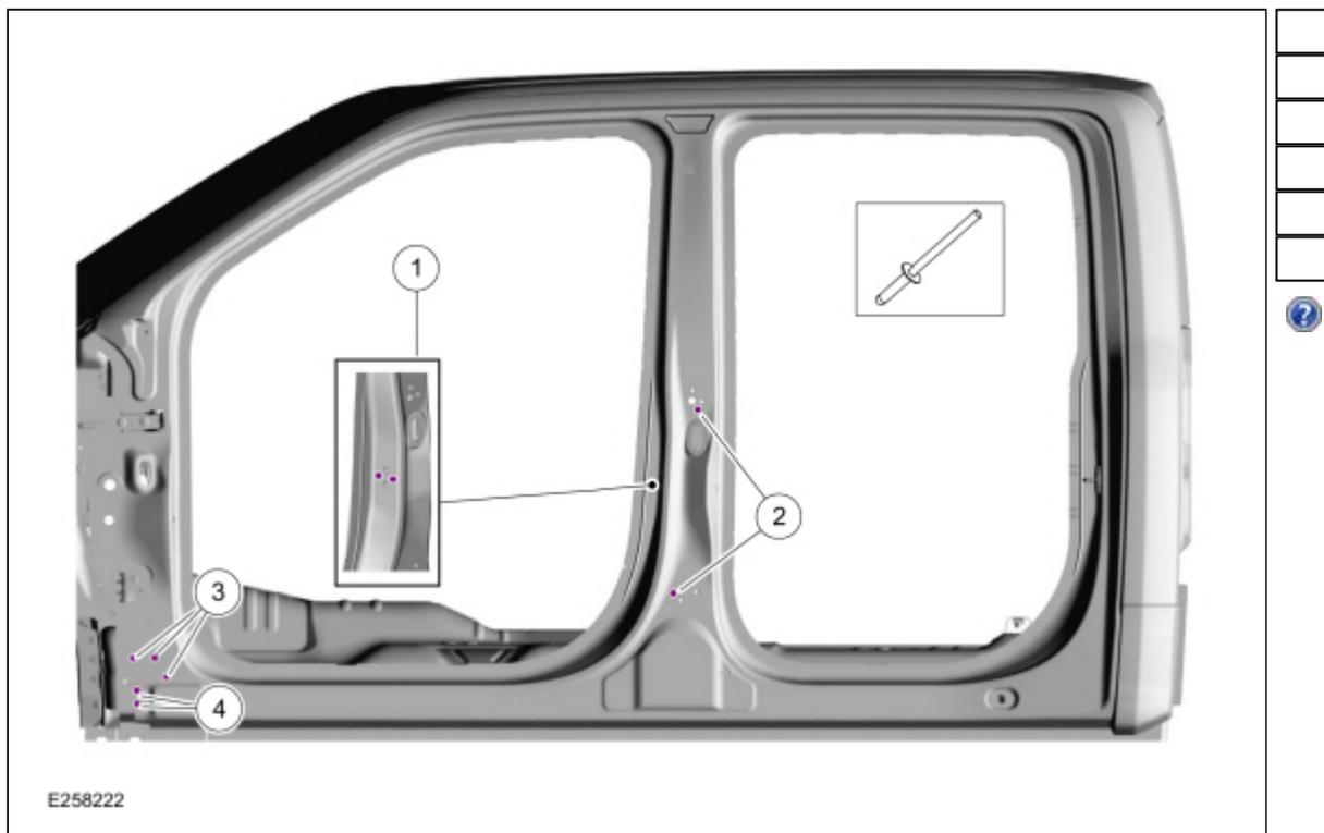
26. **NOTE:** SPR fasteners may be replaced with solid rivets or blind rivet fasteners after enlarging hole to 6.5 mm.
