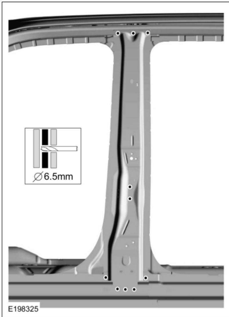
15. Install blind rivet fasteners in B-pillar reinforcement.
