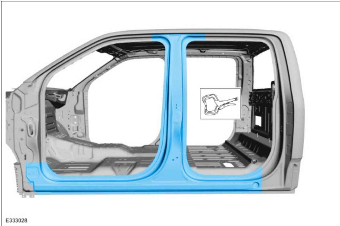
22. Complete the backer plate attachment at all sectioning joints.
