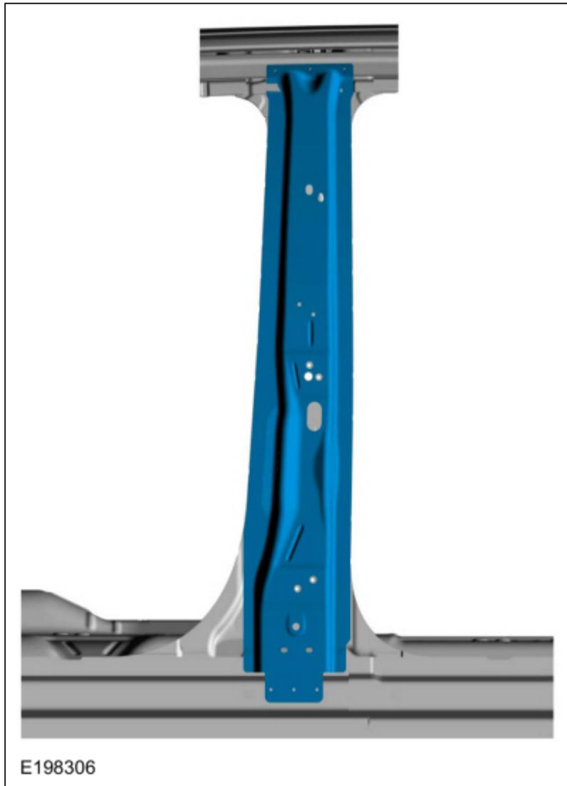
15. Remove the SPR fasteners in the rocker panel inner reinforcement.
