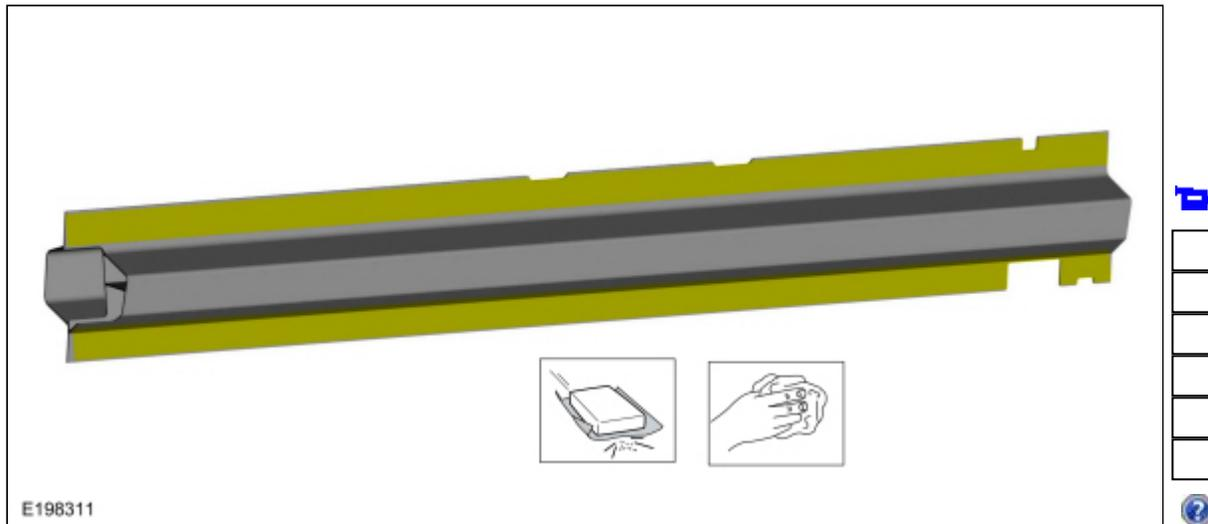
4. Apply adhesive to the front rocker panel inner reinforcement mating surface.
