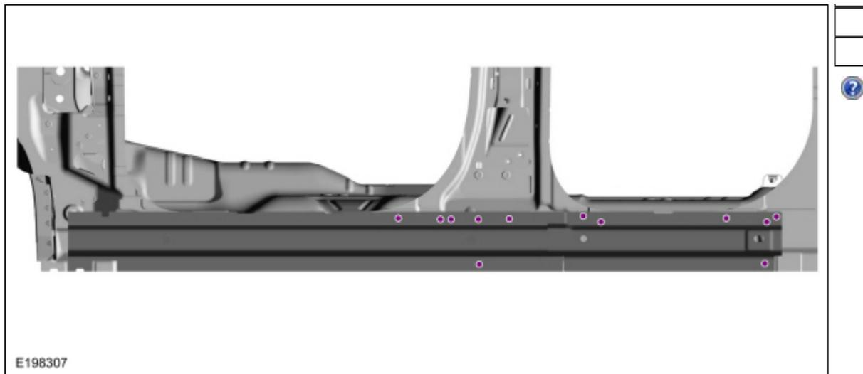
16. Remove the rocker panel inner reinforcement.
