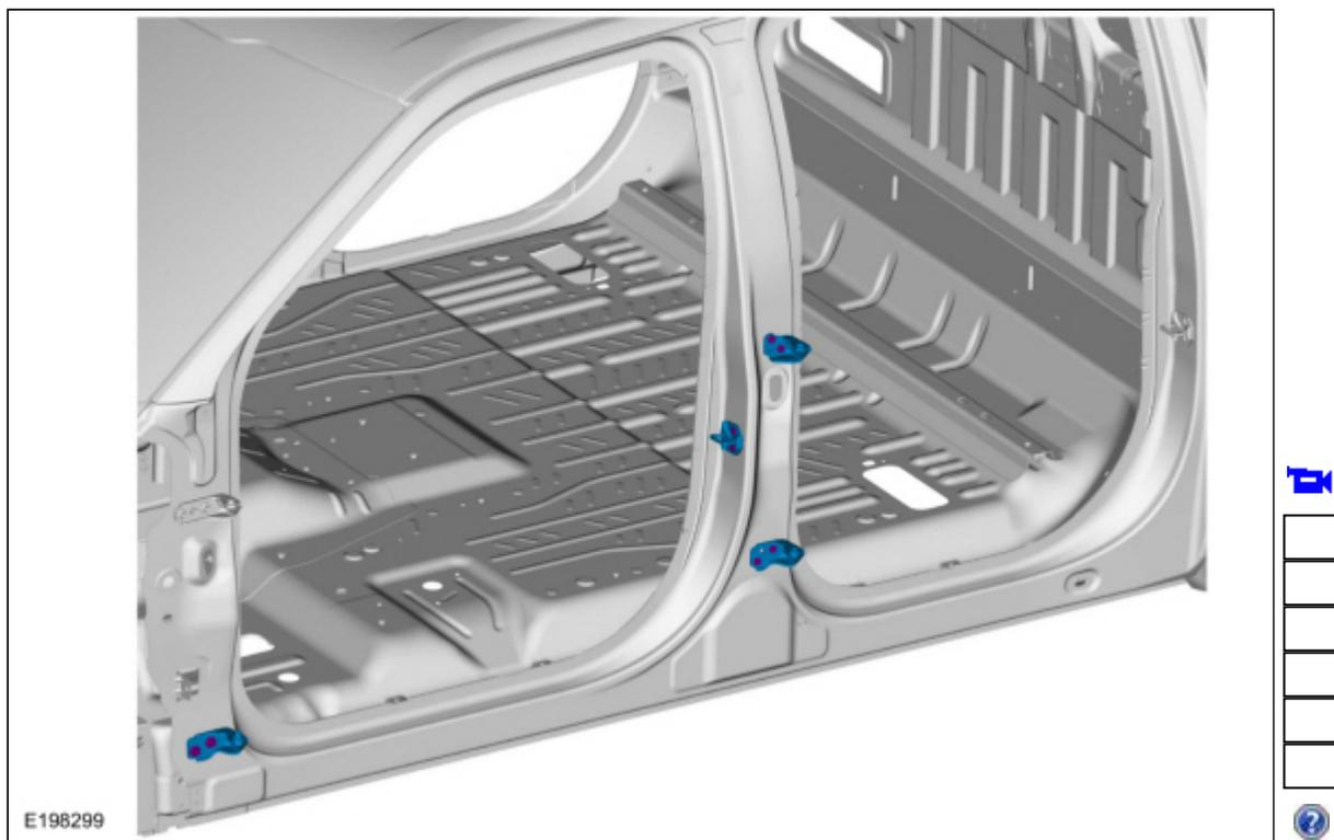
7. Remove the front and rear door scuff plates and front and rear door opening weather strips.
