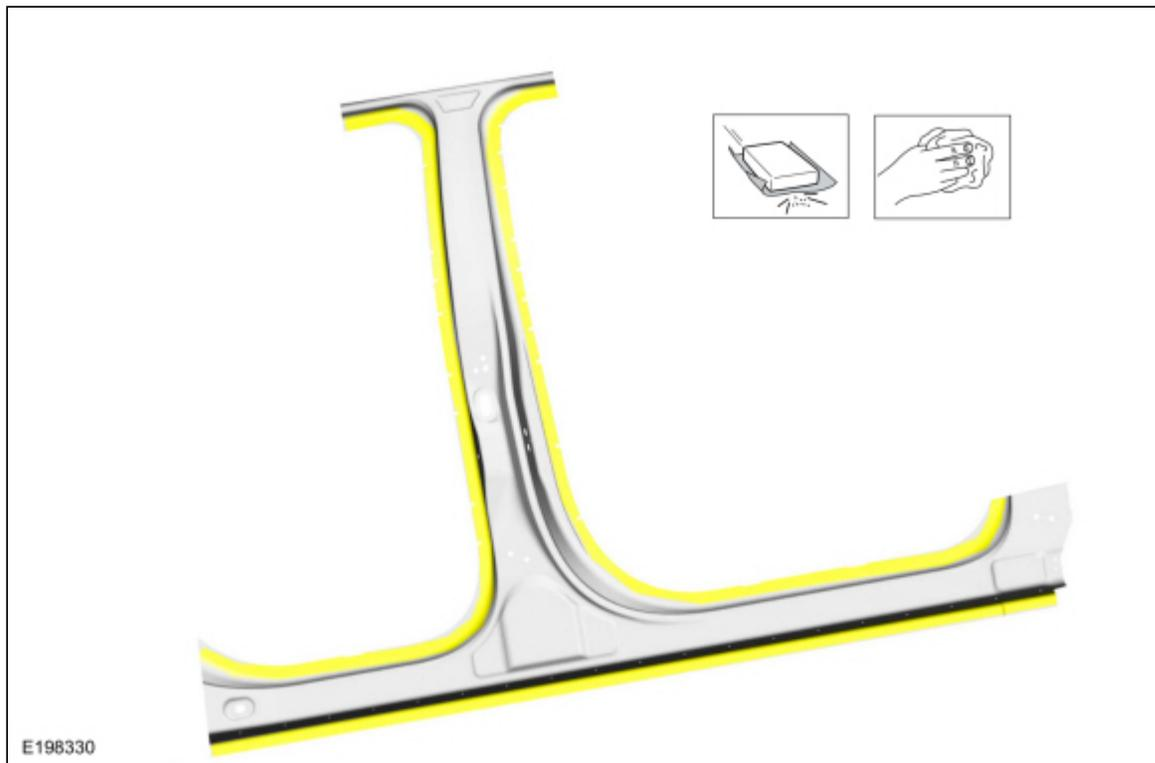
19. **NOTE:** The use of a backer plate when creating butt weld joints will produce a stronger and more uniform repair.
