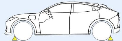
2. Put the vehicle into Park position and ensure the parking brake is engaged.
